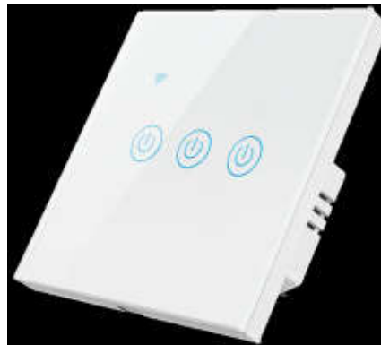
Regular color: white / black / gold... Input voltage: 100-240VAC 50 / 60Hz Network mode: ZigBee Rated power: 600W Switch (Zero Wire) European Standard / British Standard / National Standard ZigBee Touch DS-111-3
