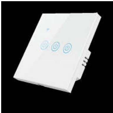
Conventional Color: White / Black / Gold... Input Voltage: 100-240VAC 50 / 60 Hz Networking Mode: WiFi Rated Power: 600W + Bluetooth) dual-mode zero fire version European / British and national standard universal WiFi touch switch (WiFi DS-101Y-3
