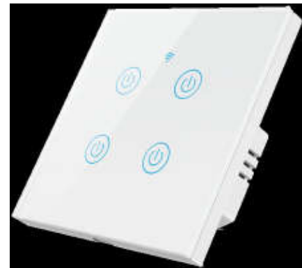
Regular color: white / black / gold... Input voltage: 100-240VAC 50 / 60Hz Network mode: ZigBee Rated power: 600W Switch (Zero Wire) European Standard / British Standard / National Standard ZigBee Touch DS-111-4
